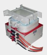
Transformer with integrated reactor Rated power 85 kVA @ 50 Hz Primary Winding 1000 V / 49 A Secondary voltage 345 V / 143 A Insulation Class H Dimensions 450x380x430 mm Weight 235kg
